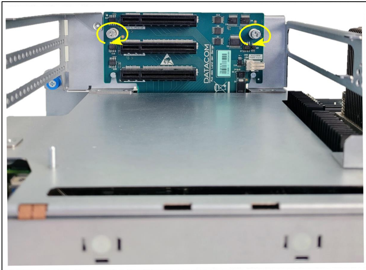
Figure 88: Riser Card Screws fixing
