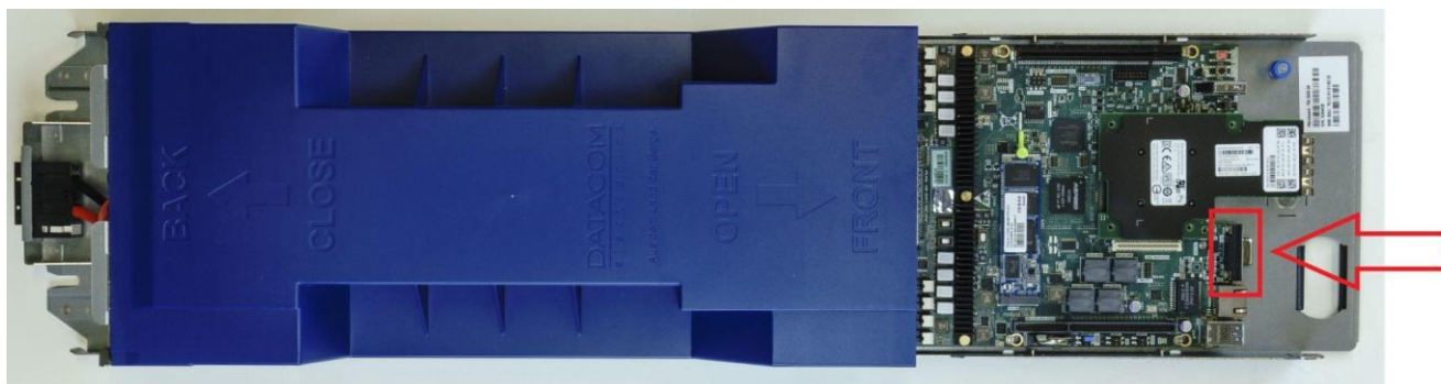
Figure 12: DM-SV01 VGA location
