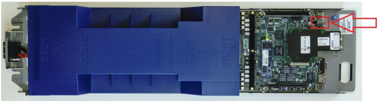
Figure 18: Debug Connector Location
