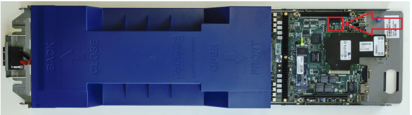
Figure 103: TPM module location
