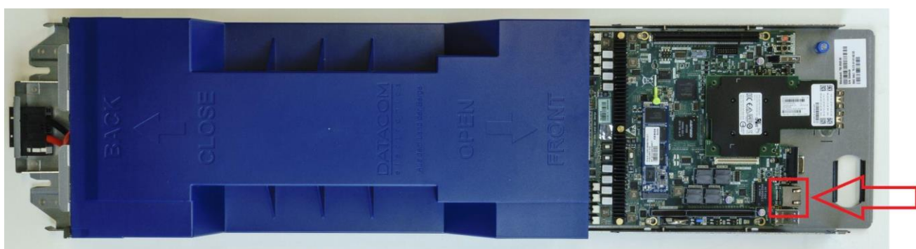
Figure 16: DM-SV01 LAN Connector location
