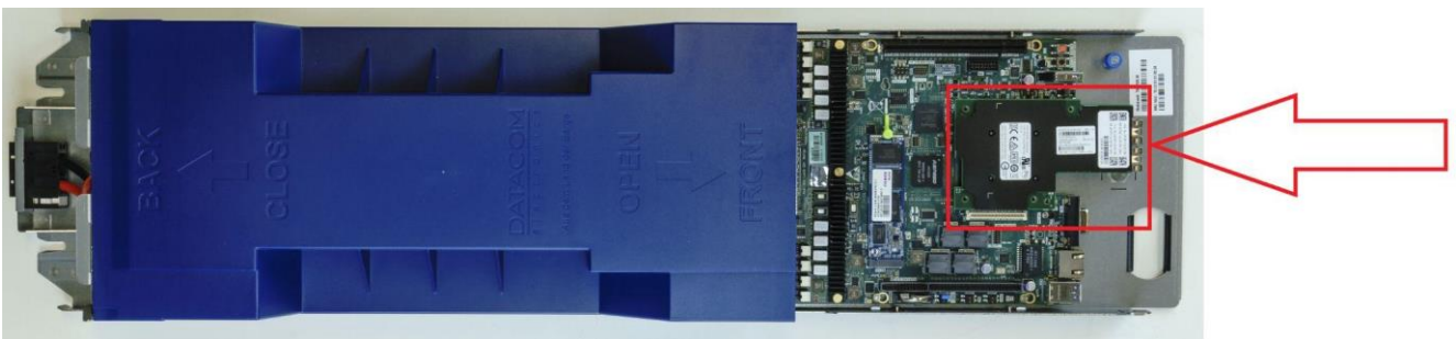
Figure 25: Mezzanine slot location
