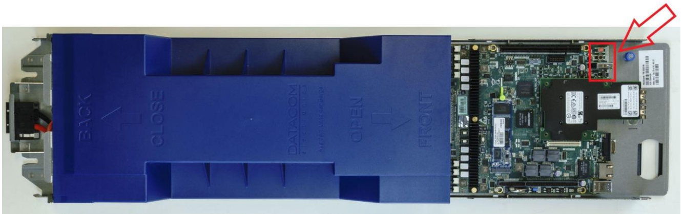
Figure 111: DM-SV01 LEDs location - top view
