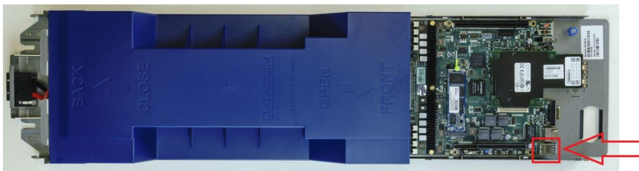
Figure 14: DM-SV01 USB 3.1 ports location
