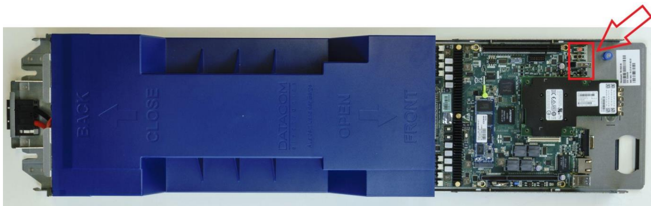
Figure 10: DM-SV01 LEDs location
