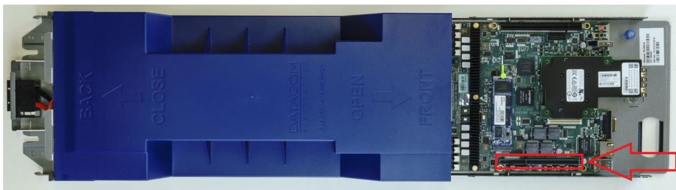
Figure 27: Expansion slot x24 location
