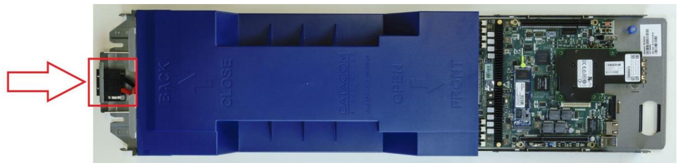
Figure 19: Power connector location
