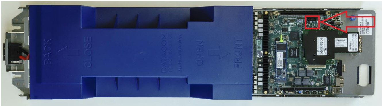
Figure 22: TPM module location
