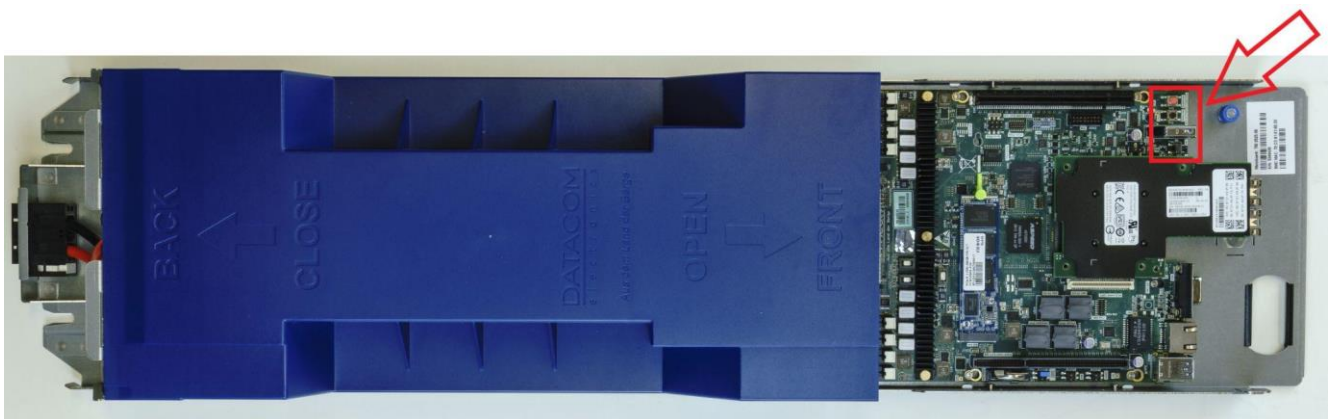
Figure 8: DM-SV01 buttons location
