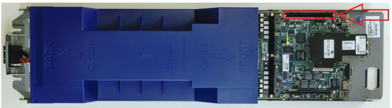
Figure 39: expansion slot x16 location
