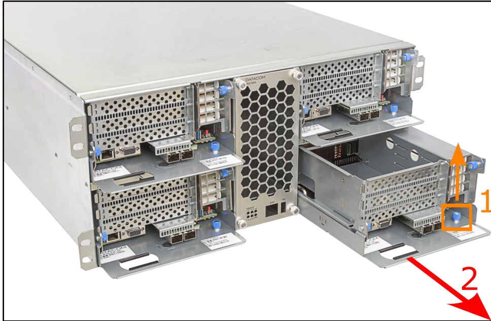
Figure 65: Removing DM-SV01 from the DM1904
