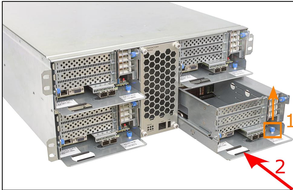
Figure 64: Inserting the DM-SV01 into the DM1904
