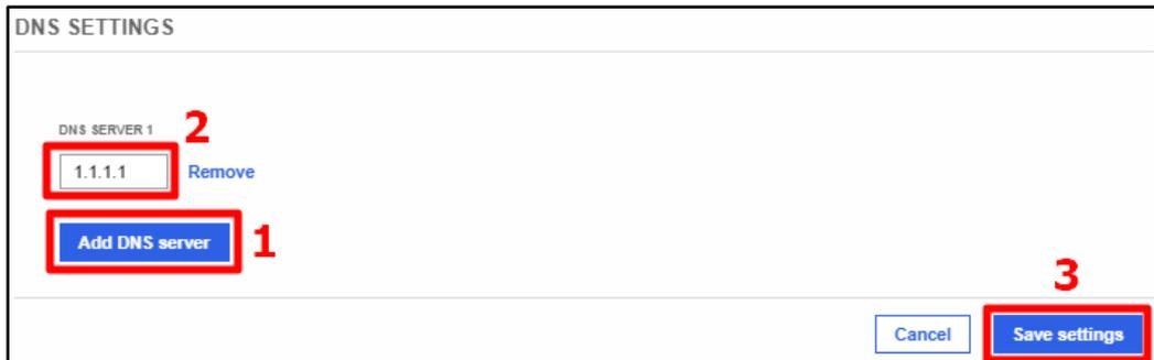
Figure 127: BMC network settings - configuring DNS server
