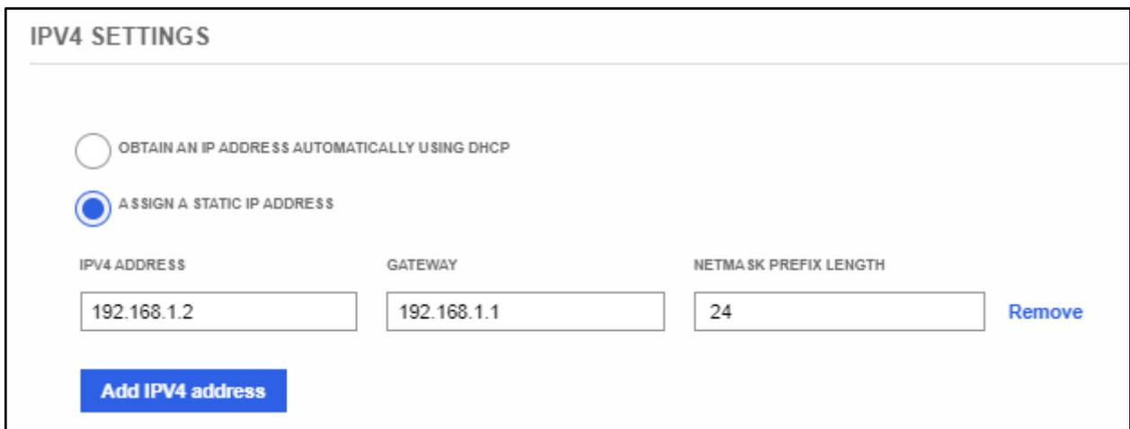
Figure 36: BMC network settings - configuring static IPv4 entries
