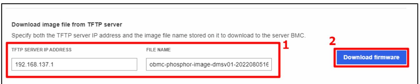
Figure 40: Firmware menu - configuring TFTP server for file transfer
